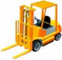
In the absence of a sling bar, in some cases unloading can also be done by using suitable **forklift trucks**. To avoid damaging the panel or even breaking the package, in these cases the distance between the forks and the width of the lifting equipment must take into account the **length of the pack**, its **weight**, as well as the **panel thickness**.
