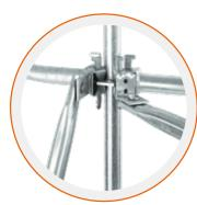
The SM8 system is made of vertical elements, as uprights, that have every 500 mm an octagonal node. Each node has 8 shaped holes into which insert the connections elements welded on ledgers, diagonals and beams.
